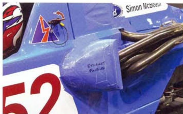
A fairing positioned ahead of the exhaust actually seemed to cause a small drag increase
