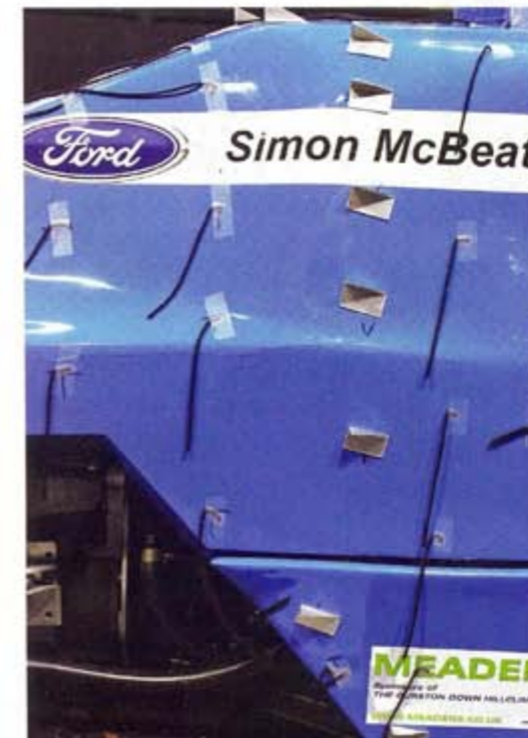
Vortex generators on the engine cover and lower flanks were aimed at reducing the car's wake but actually added some drag
