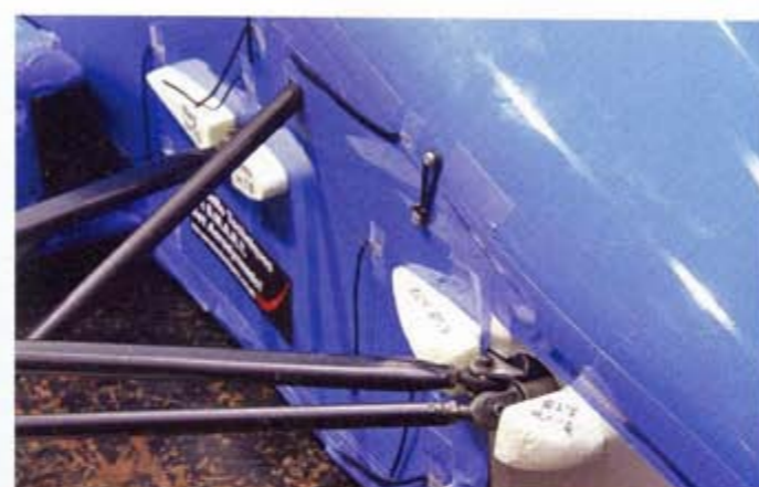
Shaped foam suspension mount fairings provided some help in reducing the drag
