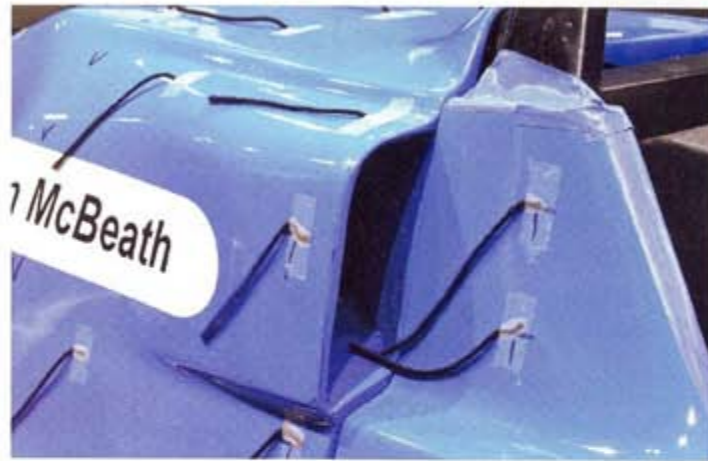
The object of one of our experiments was to find out if the engine inlet duct created drag
