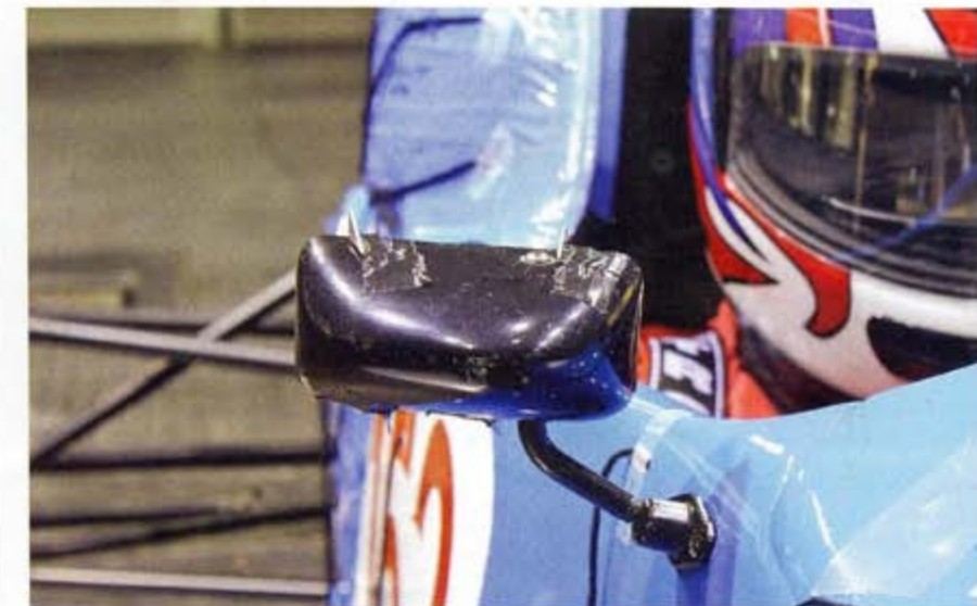
Small vortex generators were fitted on the car's mirrors with the object of reducing the size of their wake
