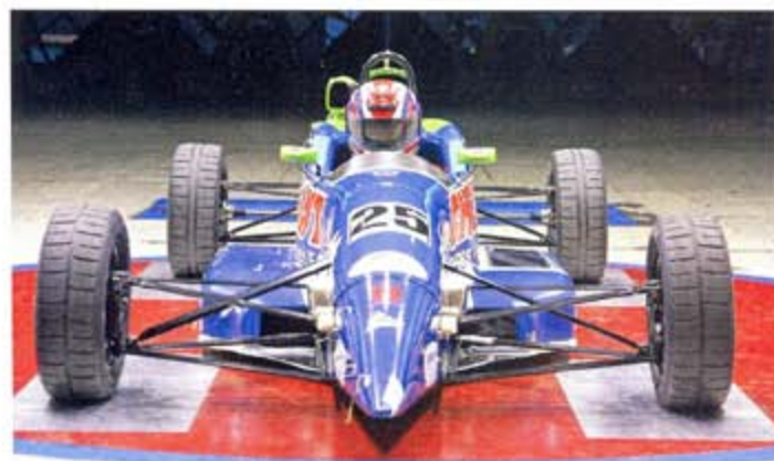
The Spectrum we tested back in 2007 had lower overall drag than the earlier Swift despite the presence of those wider sidepods, which house lateral intrusion structures
