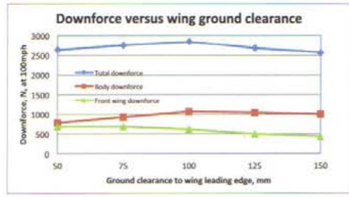
Figure 17: car body, front wing and total downforce vs wing ground clearance
