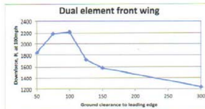
Figure 3: downforce vs ground clearance on a dual-element wing
