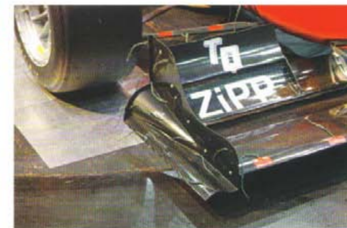
Dj Firestorm 1300mm front wing plus 100mm VEEPs
