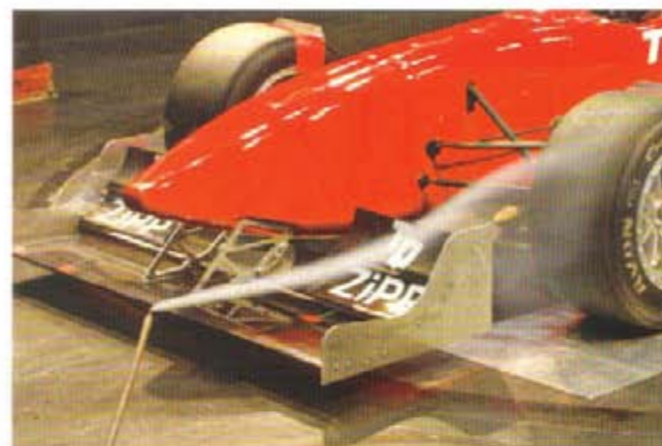
Dj Firestorm front wing at 1300mm span plus thin end plates
