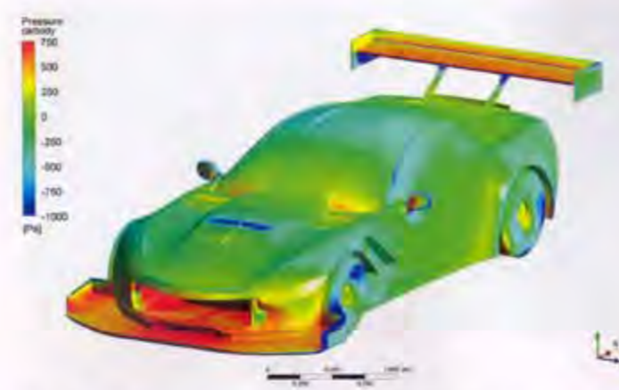
Figure 18: With wide splitter a near maximum wing angle was needed for aero balance
