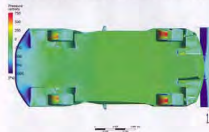
Figure 12: The first front diffuser increased splitter downforce but needed optimising
