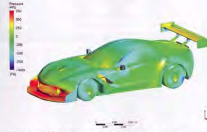
Figure 11: Here the wheel arch extractor can be seen aft of the front wheel
