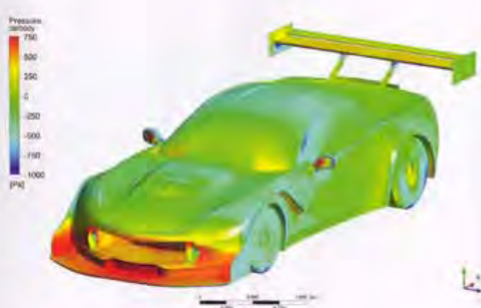
Figure 7: The 2017 racecar's more effective splitter produced some useful downforce
