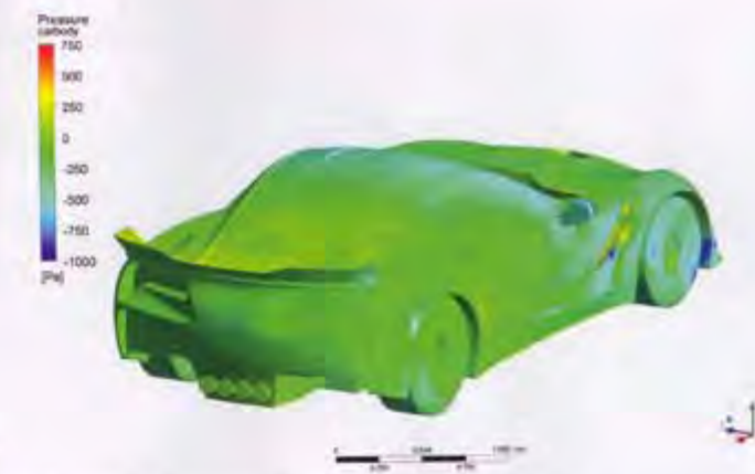
Figures 1 and 2: The pressure highs and lows on the road model of the Corvette go some way to revealing the sources of drag, lift and downforce in the car
