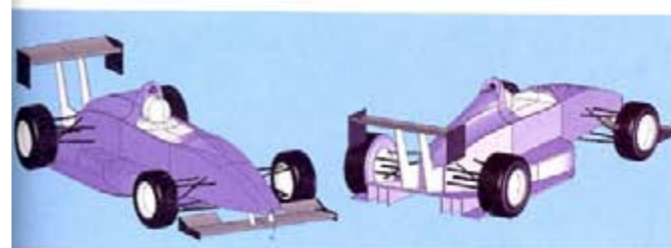
CAD Figure 1: The datum CAD model with single element, 1000mm span, 300mm chord rear wing. The racecar has been 'modified' for the purposes of this aerodynamic study
