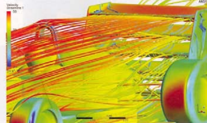
CFD-7: The airflow to each successive lower tier can be seen here to be compromised more than the one above. Yet multiple tiers can offer potential performance advantages, though that depends very much on the application. This is similar to the Katz plot
