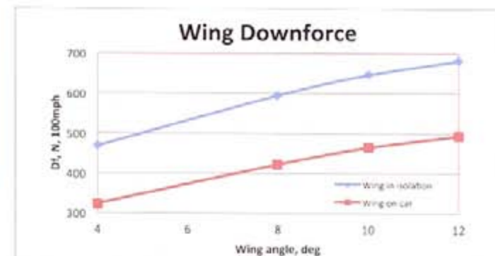
Figure 2: Wing downforce in isolation versus the performance when fixed on the car
