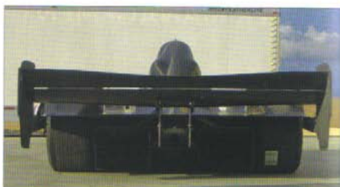
Rear shot gives a clearer idea of the wing’s low position on the Dauntless Racing Stohr WF1 (Courtesy: Dauntless Racing)
