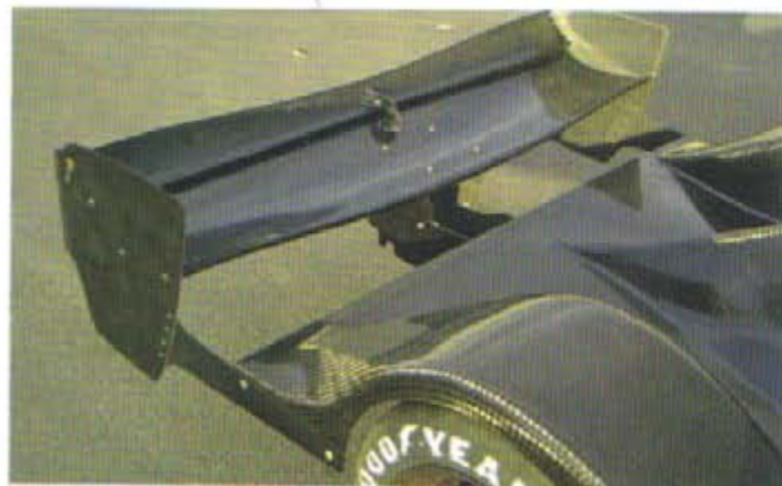
The Dauntless rear wing has been shaped to work with the flows coming off the car (Courtesy: Dauntless Racing)
