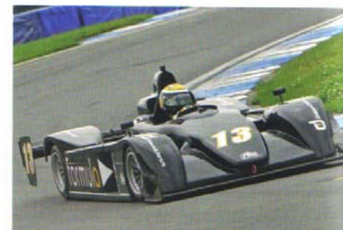
This UK-based Speeds runs a Dauntless wing and a splitter devised with Dauntless assistance (Courtesy: BookaTrack.com Ltd)
