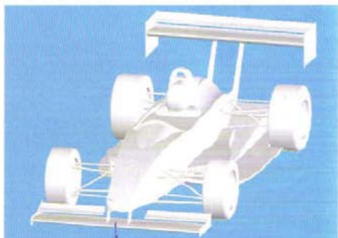
CAD 5: the single-seater model with dual-element front and rear wings
