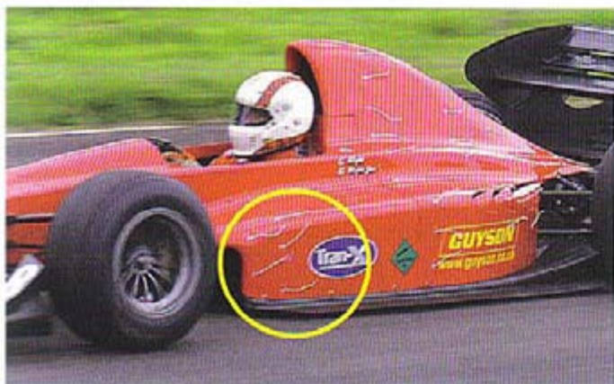
Using basic wool tufts on your racecar can be very revealing. At high speed (above left – indicated by the low ground clearance) the tufts on the front of the sidepod trail backwards as you might expect, whereas at low speed (above right – with greater ground clearance visible) the same tufts show reverse flow
