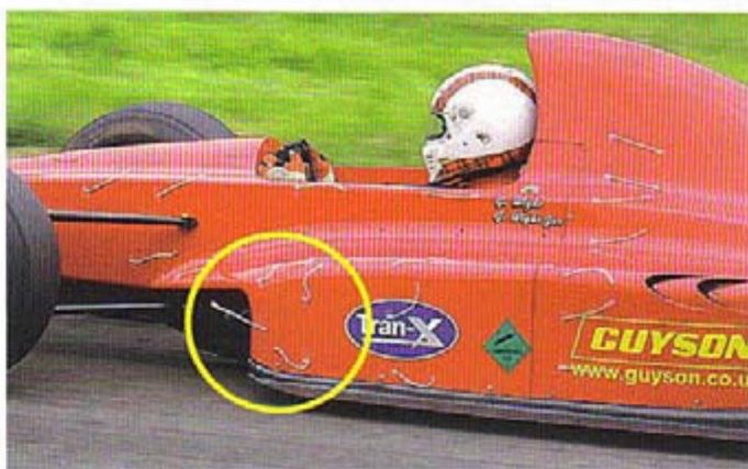
Using basic wool tufts on your racecar can be very revealing. At high speed (above left – indicated by the low ground clearance) the tufts on the front of the sidepod trail backwards as you might expect, whereas at low speed (above right – with greater ground clearance visible) the same tufts show reverse flow
