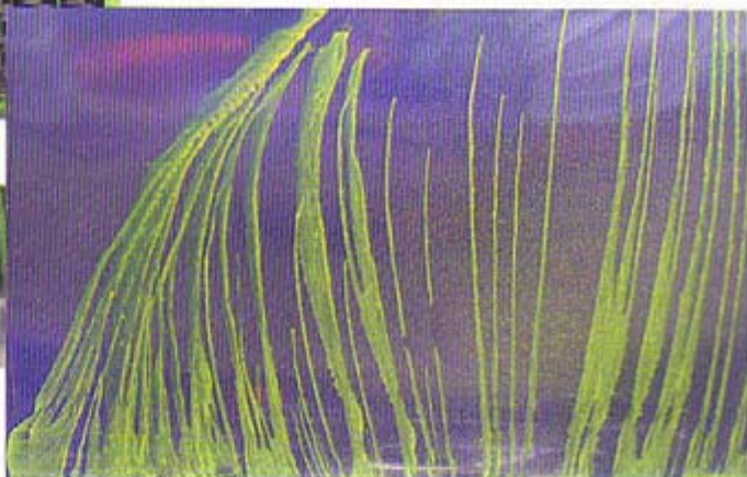
Flow visualisation fluids can be very revealing. The central mounting structure is having a very adverse effect on the flow along the underside of this wing (the wing leading edge is at the bottom of the picture)
