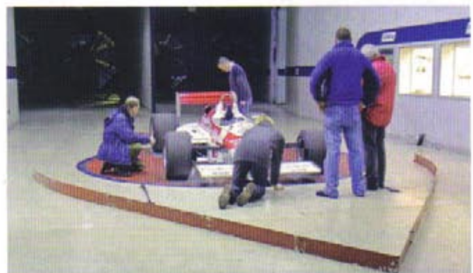
Setting the car up on the load cells and aligned with the airflow is crucial
